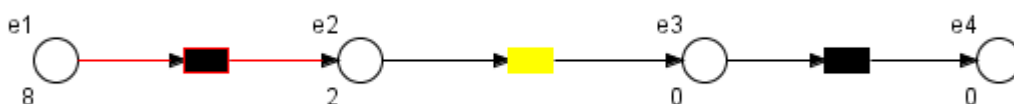
Figure 91. Process state indication in CI Player, from left to right: firing , waiting and not-firing
